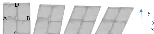
Figure 2: Automatically generated unit cell models with shear angles of 0^\circ , 10^\circ , 20^\circ and 25^\circ relative to the y-axis.
